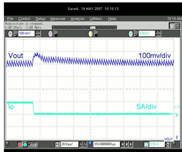
Figure 27. Load Transient – Load Release
