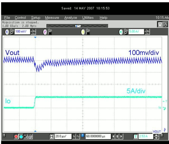
Figure 26. Load Transient – Load Step Up
